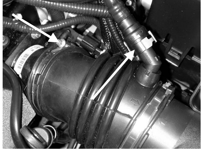
b) Release the fitting on the inlet pipe nipple. Loosen the hose clamp at the throttle body.
