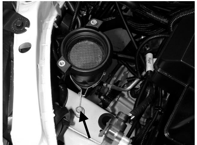
d) Remove the upper air box and the bolt in the frame rail. Release the metal clamp from the Mass Air Flow (MAF) sensor housing.
