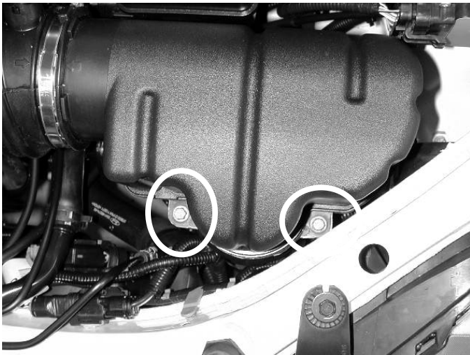
c) Loosen the two bolts that secure the upper air box.
