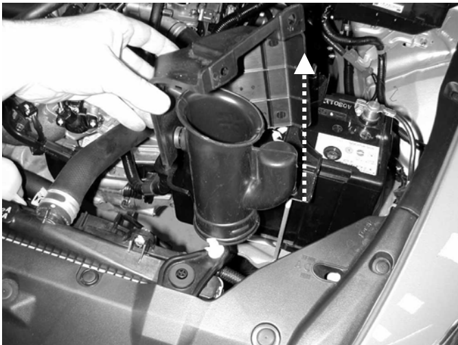
i) Pull upward on the plastic cover to remove the resonator box intake tube.
