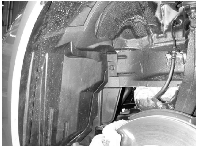
j) From inside the driver-side wheel well, remove the fastener shown in the picture.
