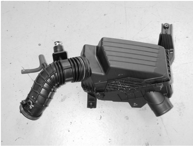
g) Carefully remove the air box assembly from the engine bay.
