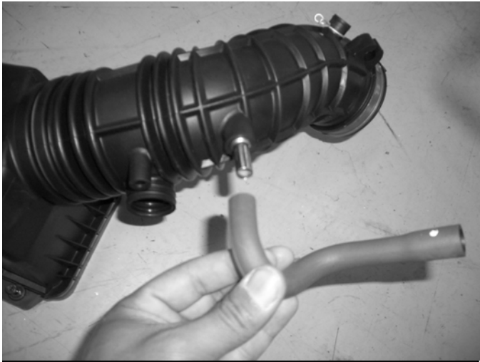
f) Remove the small hose from the factory intake system.
