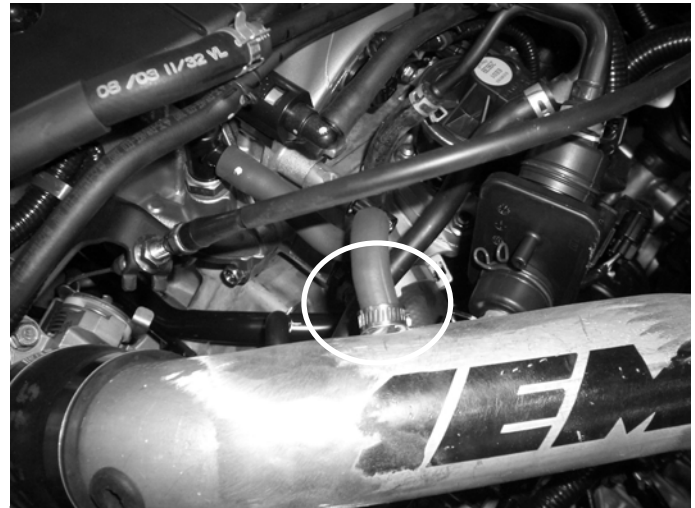
g) Re-install the small hose with the AEM intake system. Use a \frac{3}{4} " hose clamp to secure it on the small nipple on the intake pipe.
