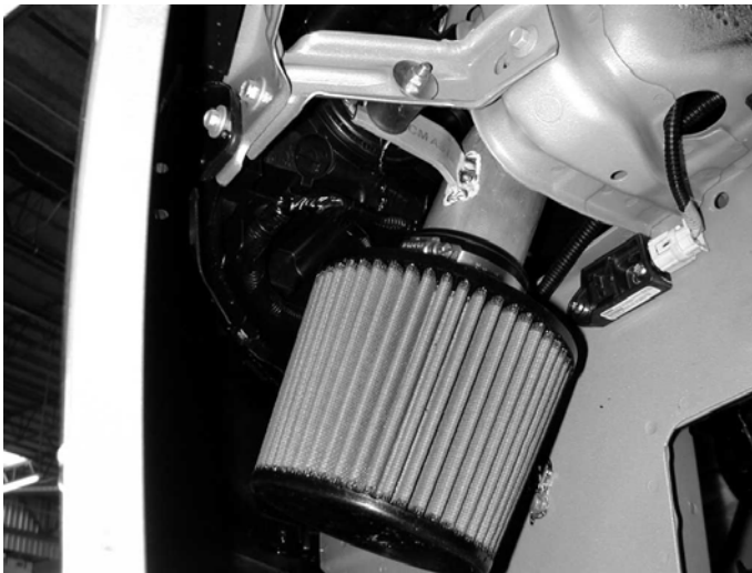
h) Install the filter on the end of the intake pipe and tighten the hose clamp.
