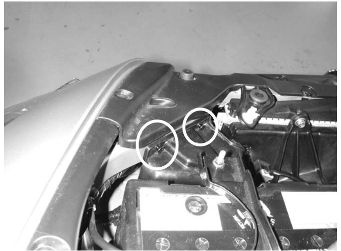
h) Remove the two fasteners holding the plastic cover in front of the battery.
