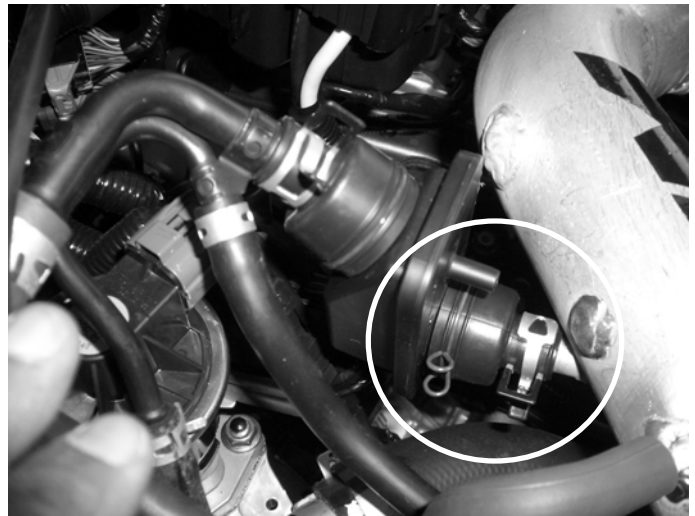
i) Attach the Oil trap coupler to the oil trap and secure with the stock clamp. Attach the small end to the inlet pipe and secure with provided spring clamp.
