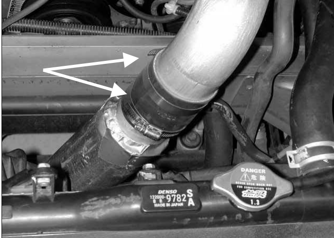
i) Using the 2.75" Silicone Hose and two hose clamps supplied, attach the Upper and Lower Intake pipes together.
