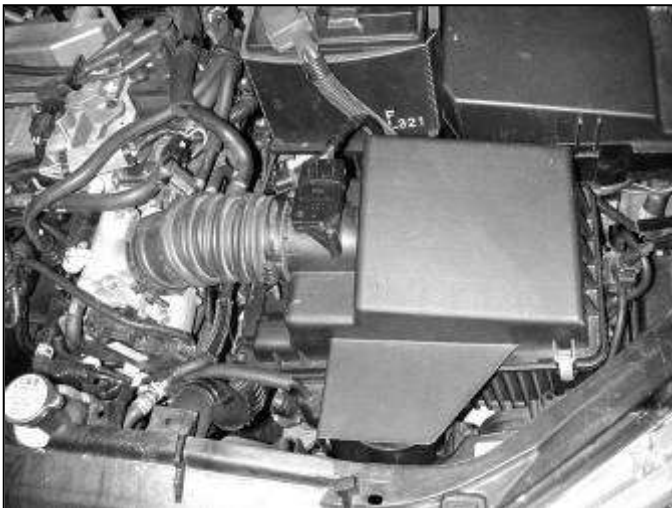
a. Stock air box system installed.
