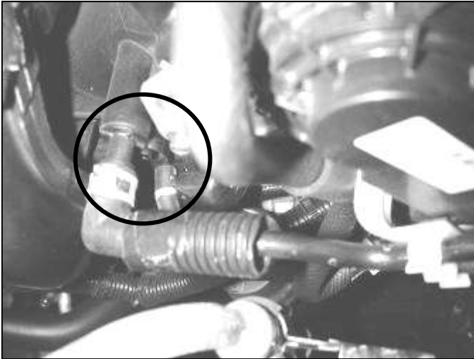
b. Pull vacuum hose off nipple on the intake manifold.
