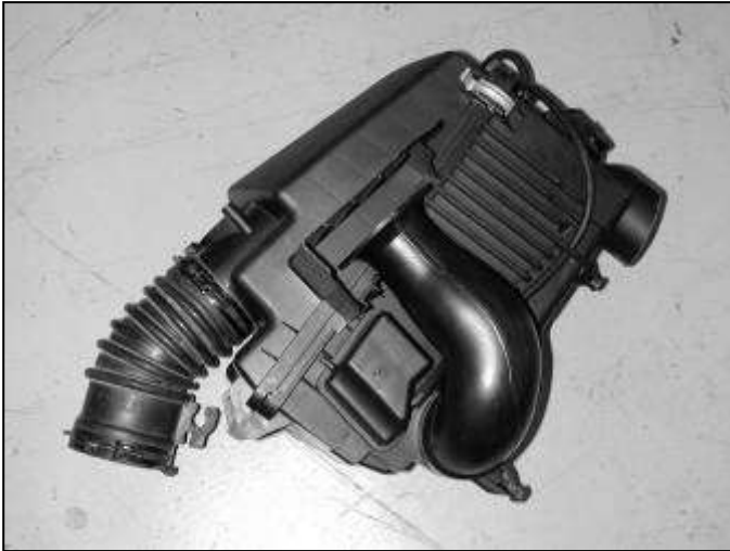
g. Pull the air box up and out of the engine bay.
