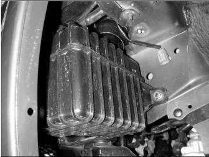
m. Remove the three nuts that secure the lower air box to the vehicle.
