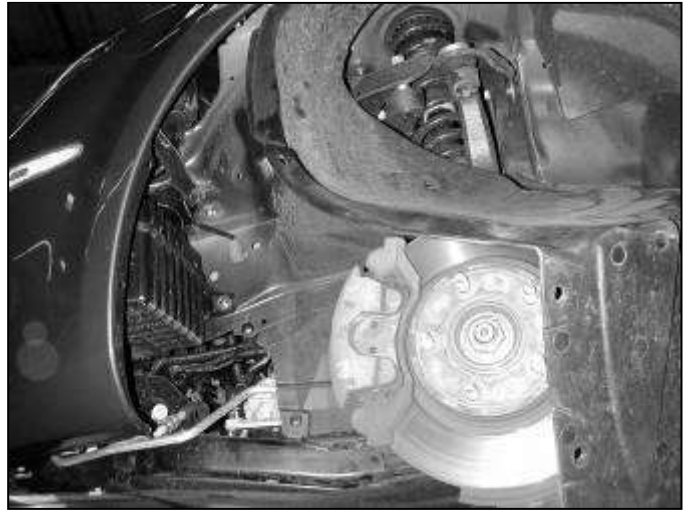
l. Partially remove the fender liner as shown.
