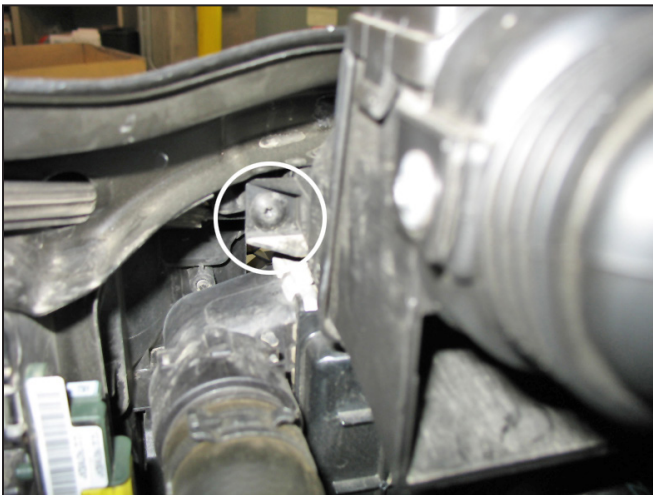
c. Remove the two torx-head screws securing the inlet duct to the radiator support. Remove the first screw shown above.
