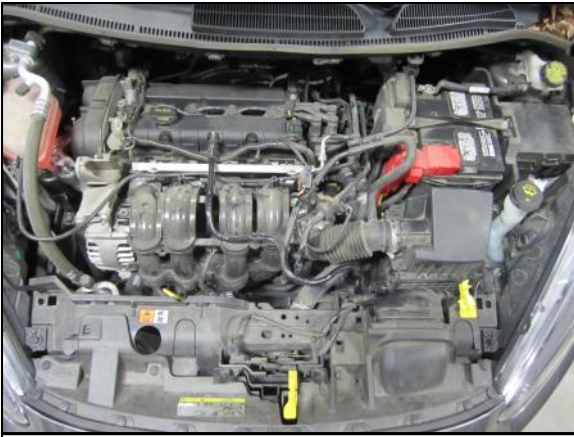
Stock Intake Installed
