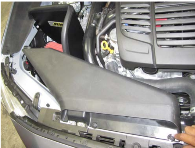
m. Reinstall stock air duct and plastic mounting clips. Ensure clearance with filter and adjust position of tube if necessary.
