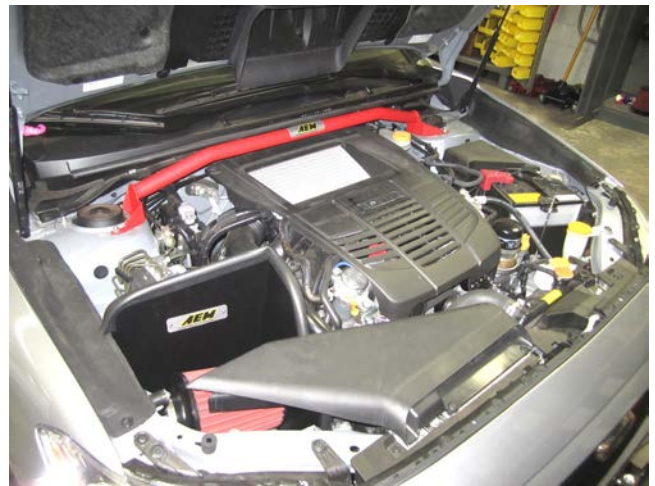
n. AEM intake installed.
