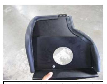
d. Install the supplied edge trims (102494 & 8-4013) onto the outer part of the heat shield.
