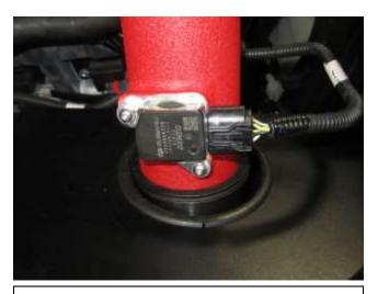
n. Plug in the mass air flow sensor connector that was detached in 2b.
