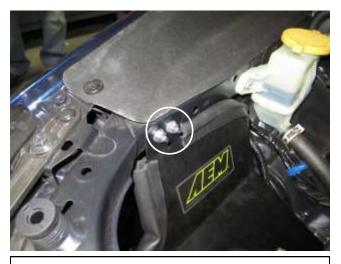
i. Re-install the nuts that were removed 2c) and tighten.
