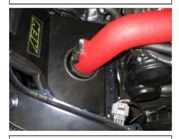
h. Install the filter, heat shield, and tube assembly into the vehicle.
