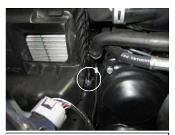
d. Remove the bolt that secures the air box to the engine bay.
