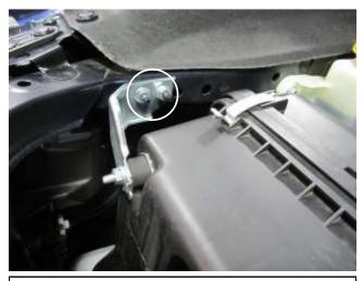
c. Remove the two bolts on the fender that secure the bracket. These will be re-used.
