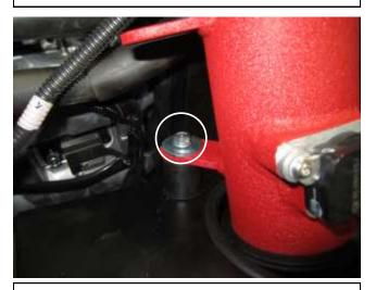
I. Align the bracket with the rubber mount and tighten the washer (08160) and nut (444.460.04).
