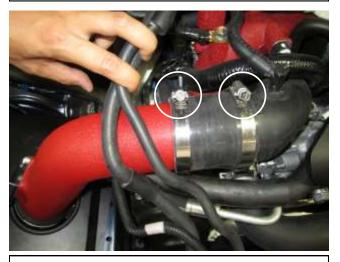
k. Install the supplied coupler (5-275) and tighten the two hose clamps (9444) onto the AEM intake tube and compressor inlet tube.
