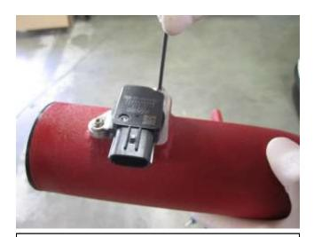
a. Install the mass air flow sensor that was removed in2f) into the AEM intake tube with the supplied hardware(1-2051) with 4MM Hex Key.
