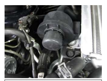
b. Install the supplied cap over the sound tube diaphragm (8-206).
