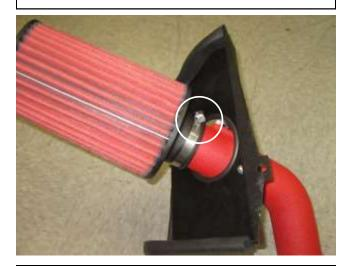
g. Install the AEM filter onto the AEM intake tube through the heat shield and tighten the hose clamp (9448)
