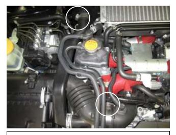
e. Loosen the hose clamps at the sound tube and the stock intake tube. Then remove the complete air box from the vehicle. **NOTE:** Do not discard your stock equipment.
