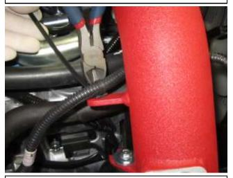
m. Secure the mass air flow sensor loom to the AEM intake tube with supplied push-in zip tie.
