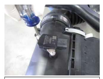
f. Remove the mass air flow sensor from the stock air box. This will be reused in 3a.
