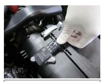
b. Depress the tab on the mass air flow sensor plug and disconnect it from the sensor.
