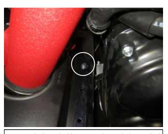
j. Secure the heat shield to engine bay with the supplied bolt (1-2038) .
