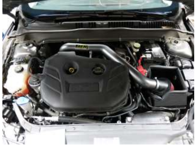
AEM INTAKE INSTALLED
