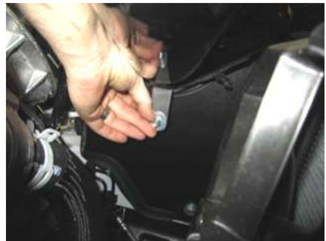
j. Install washer and nut on the bracket on the underside of the intake tube.
