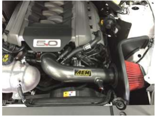
p. Finished installation of AEM Intake System.
