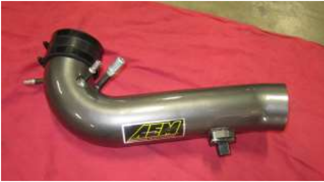
e. Assemble the intake tube components as shown above including the hose, clamps, and MAF sensor.
