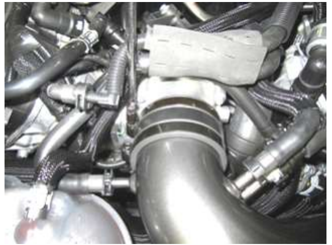
h. Lower the tube into the vehicle aligning the filter end in the heat shield first and then slipping the hose over the throttle body. Push on all lines as shown above until they click on securely. Ensure that wiring harness remains in front of the bracket on the bottom of the tube and reconnect to the MAF sensor.
