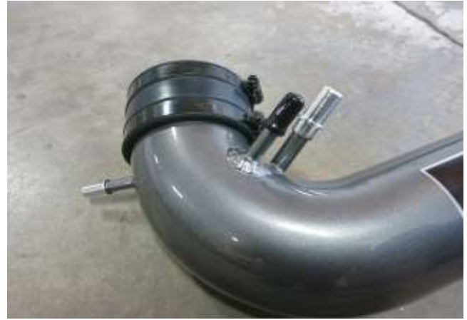
f. For models with only one PCV line, use the supplied vacuum cap to cover the extra nipple.
