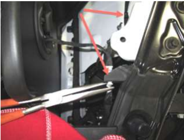
g. Release the other sensor wiring retaining clips. Pass the harness through the tube hole in the heat shield.
