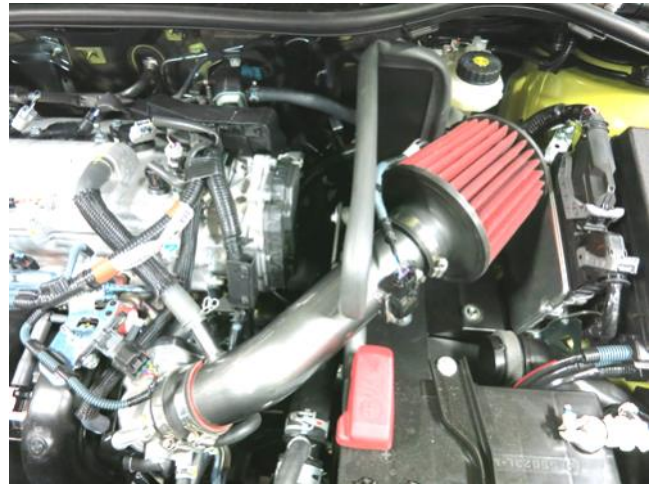
l. Reconnect the vent hose to the intake tube and tighten all hose clamps .
