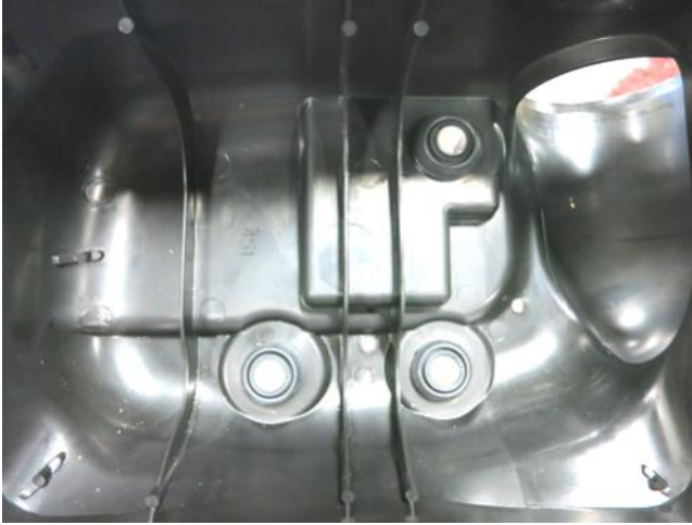
a. Remove the three rubber grommets and metal sleeves from the lower air box.
