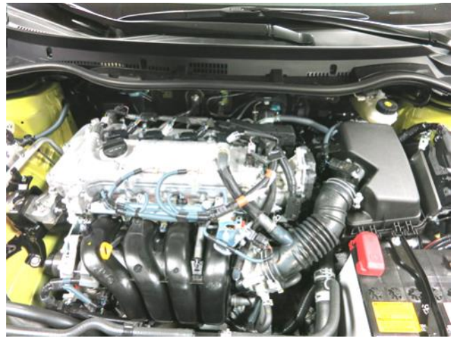
b. Remove the engine cover by gently pulling it up from the engine.
