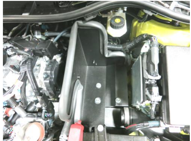
d. Drop the complete heat shield assembly into the engine compartment. Secure the wiring harness bracket to the back of the heat shield and then secure the heat shield to the engine compartment with the three M6 bolts removed in step 2 g.
