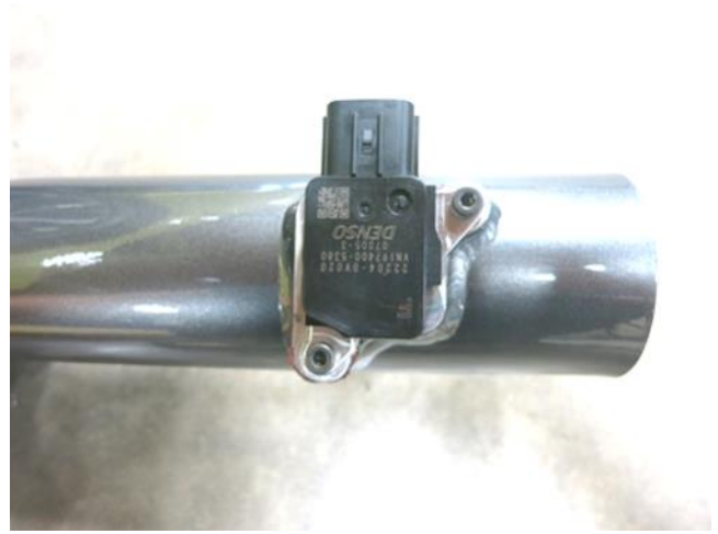
f. Remove the MAF sensor from the factory air box and transfer it onto the AEM intake tube, secure with 4MM bolts supplied.
