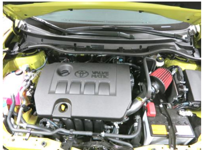
n. AEM 21-776C intake system installed.
