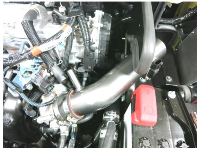
h. Install the complete intake tube assembly to the coupler and line up bracket with the rubber mounted stud.
