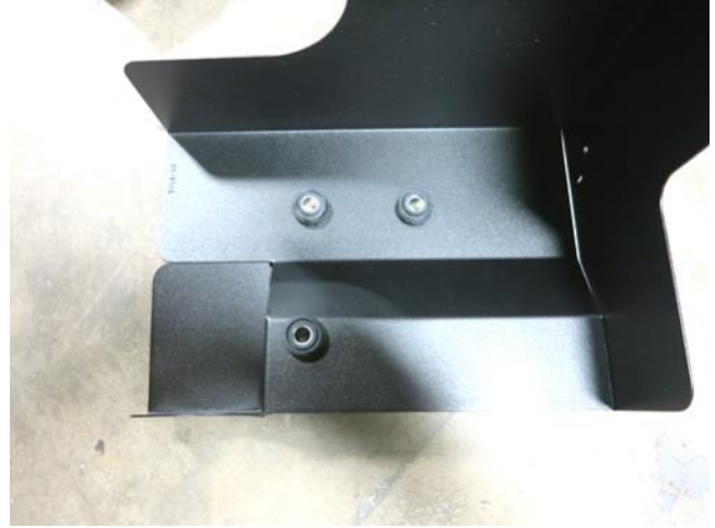
b. Install the grommets and metal sleeves onto the AEM heat shield as shown.
