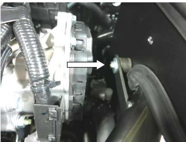
i. Secure the AEM intake tube to the rubber mounted stud with the supplied M6 nut and washer.
