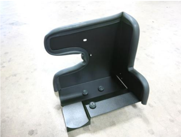
c. Install the supplied rubber edge trim on the AEM heat shield as shown.
