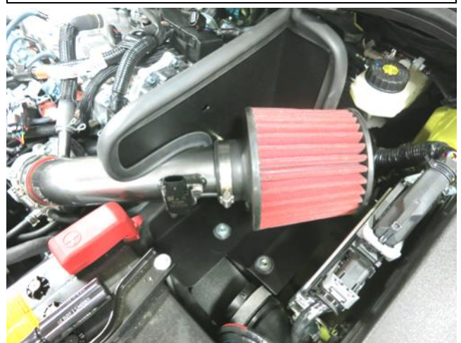
j. Install the AEM filter onto the intake tube as shown.
