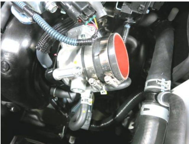
g. Install the supplied coupler and #40 hose clamps on the throttle body.
