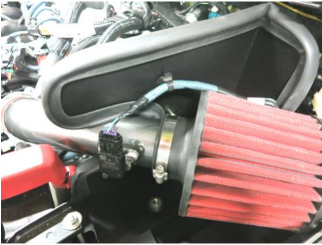
k. Reconnect the MAF sensor and secure the wiring harness clip to the heat shield as shown.
