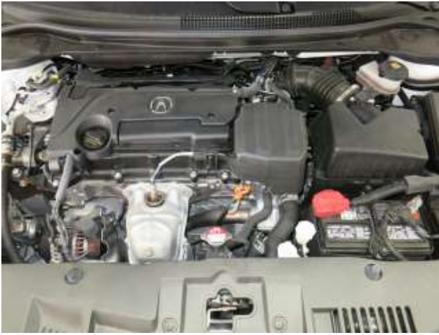
STOCK INTAKE INSTALLED
