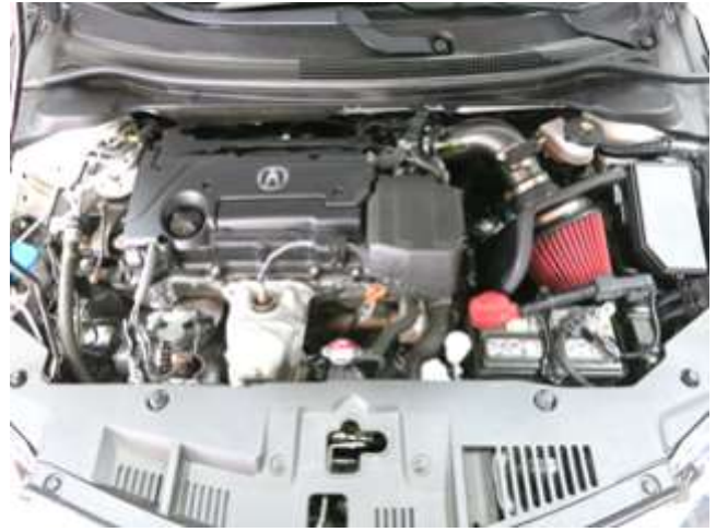
AEM INTAKE INSTALLED
