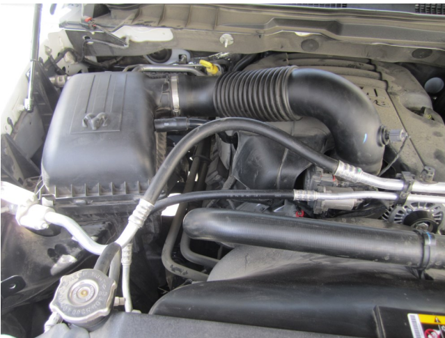
Factory air box system installed
