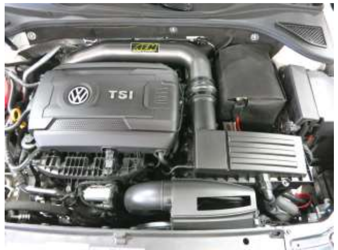
g. Finished installation of AEM Intake System.
