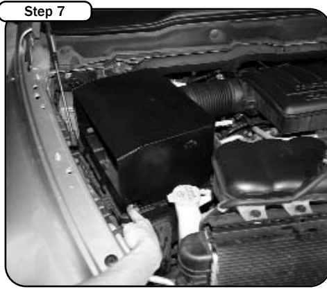
Insert housing assembly into the lower portion of the factory airbox. Secure housing with the factory airbox clips.
