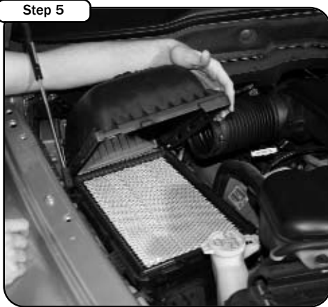
Remove upper portion of the airbox. Lift up and remove the factory paper filter.
