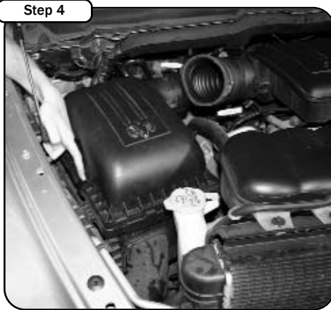
Loosen the four clips securing the upper portion of the airbox.
