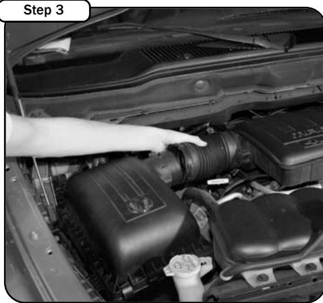
Loosen hose clamp on the air duct connecting to the airbox. Disconnect the breather hose (if equipped). Move air duct to the side
