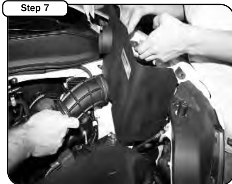
Step 7 Position the new housing inside the engine compartment. Make sure the lower mounting tab slide in the snorkel mount.
