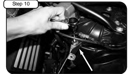
With OE T25 bolt, use to tighten new housing in to place. Tighten at bottom of housing using nut and washer provided with 10mm socket w/ extension.
