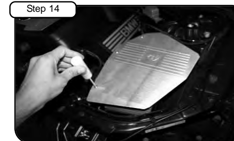
Place high FLOW filter into housing and tighten using 5/16" nut driver. Install housing cover using the 3 button head screws and tighten using 5/32" allen key.
