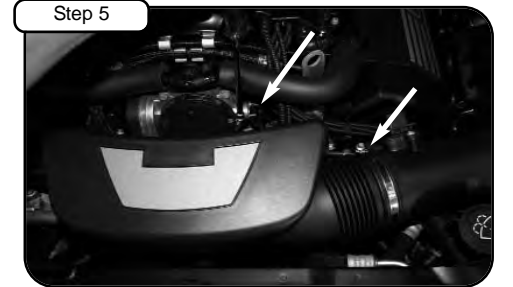
With 1/4" nut driver loosen the OE intake tube from throttle body and airbox. Remove intake tube out of vehicle.
