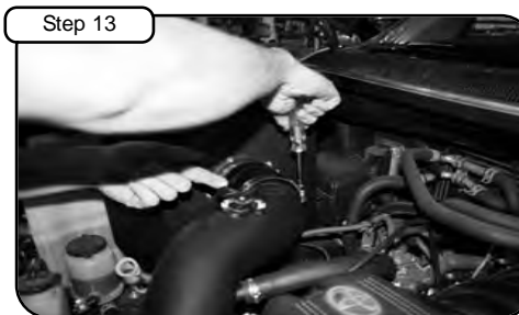
Tighten clamps at housing side using 5/16" nut driver. Re-connect MAF sensor harness.
