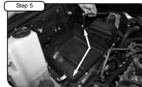
With 10mm socket or wrench loosen both bolts holding in air-box. Remove complete air-box out of vehicle.
