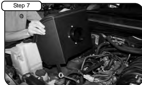
Install housing to vehicle. Use M6 screws with flat washers provided. Make sure 1/4" nylon spacer is between housing and fender when installing.
