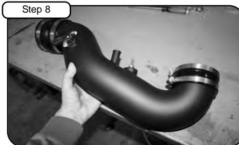
Remove MAF sensor from OE air box. Install into new tube using gasket, 1/8" nylon spacers, and M4 screws provided. Install brass nipple to tube and tighten. Install couplers with clamps to tube.
