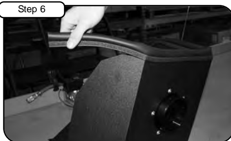
Install filter adaptor to inside of housing using 5 button head screws and wavy washers. Tighten using 5/32 allen key. Install 3/4" trim seal to housing.
