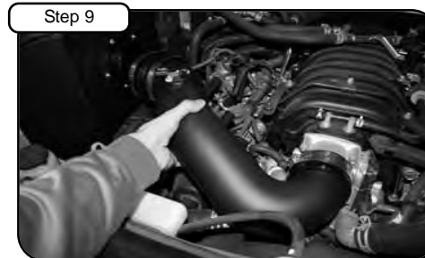
Install new tube into vehicle. Position tube to throttle body and housing. Do not tighten clamps.
