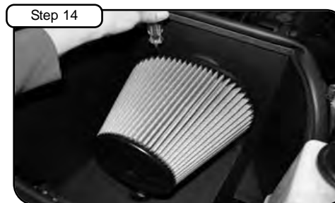
Install air filter and tighten using 5/16" nut driver. Re-install small engine cover.
