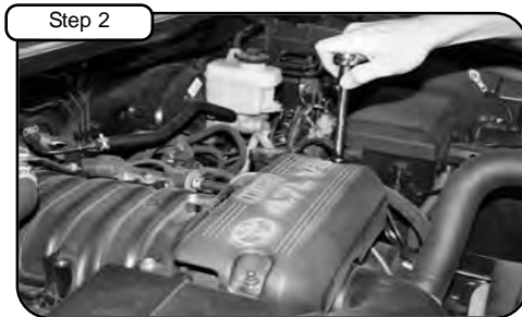
With 10mm wrench or socket, loosen bolts on engine cover. Disconnect MAF sensor harness.
