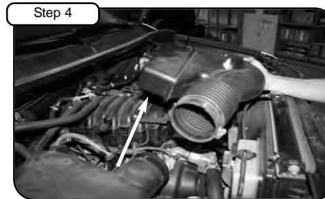
Remove OE intake tube. Un-clip upper half of air-box and remove with OE air filter.
