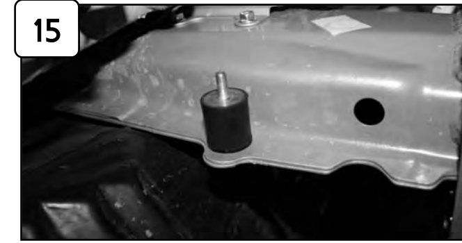
15 Install isolation mount to frame.
