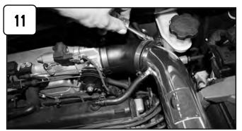
Tighten all clamps using 5/16" nut driver. Re-attach crank case line to intake tube using pliers.
