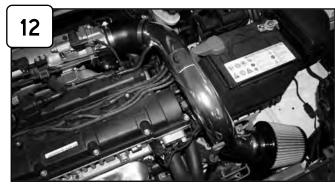
Install air filter and tighten using 5/16" nut driver. Attach pre filter to filter if desired. Your short ram intake is now complete.
