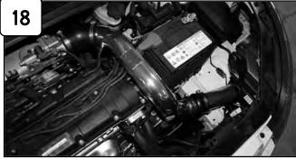
The installation of your Takeda performance intake is now complete. Please check all components and retighten if necessary. Reconnect battery terminals. Thank you for choosing Takeda!
