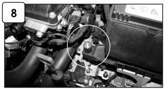
Install provided M6 isolation mount to factory air box mounting point next to battery tray.
