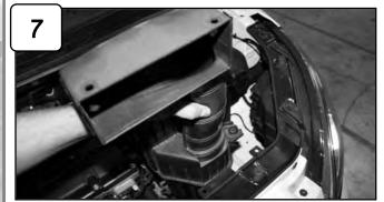
With phillips screwdriver, loosen the 2 top plastic clips on top of ram scoop and remove bottom half of air box.
