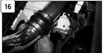
With provided flat washer and nut, tighten tab to isolation mount from step 13.
