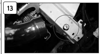
Remove air filter. Install and tighten isolation mount to frame.
