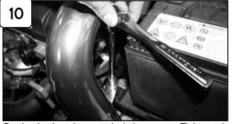
Postion intake tube on to isolation mount. Tighten tab on isolation mount using provided M6 nut and washer.
