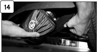
With phillips screwdriver loosen the 2 plastic clips on bottom of plastic bumper cover. Attach pre filter (if not already done) to filter and place filter inside front of driver side wheel.
