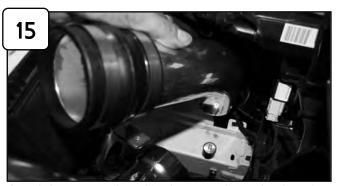
Attach hump coupler with clamps to lower intake tube. Install lower intake tube assembly. Position on to isolation mount. Slide coupler back over upper intake tube. Do not tighten.
