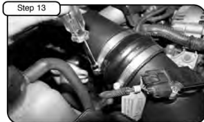
Step 13 Install hump coupling with clamps provided and secure. Tighten all clamps using 5/16" nut driver. Reconnect MAF sensor harness.
