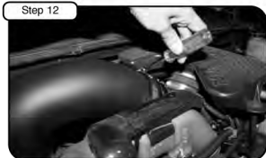
Step 12 Install 05-01072 tube to turbo side with 05-00033 reducer coupling and clamps provided and position to tube on housing. Do not tighten clamps.
