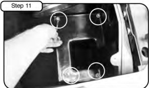
Step 11 Use the 4 bolts from step 9 and tighten housing using 10mm socket or wrench.
