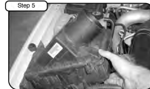
Step 5 Lift and pull air box out of vehicle.
