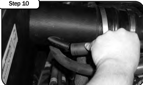
Insert the rubber breather hose into the new intake pipe. No clamps are required.
