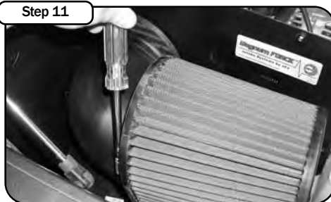
Install the pre-oiled filter in the housing and tighten down clamp. DO-NOT use any oil or grease.
