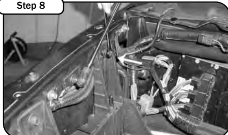
Remove the 13mm bolt on the left side of the engine bay by the hood shock. Place the assemble intake pipe and housing assembly into the factory location. Line up the plastic pins on the bottom of the engine bay with the rubber grommets and lower the housing in. Line up the mounting hole on the side of the housing and reinstall the 13mm bolt
