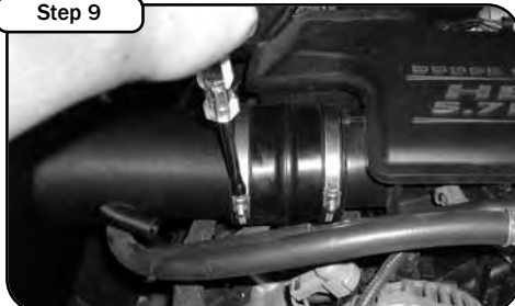
Slide the urethane coupler over the inlet and tighten the hose clamps.
