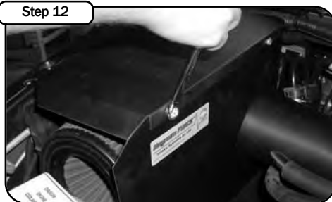
Install the housing lid to the housing. Fasten lid to housing with the supplied button head screws.
