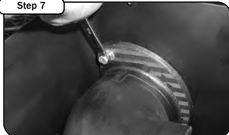
Insert the new intake pipe thru the entry hole on side of the housing. Bolt the flange on the pipe to the housing using the supplied nuts and bolts. (Make sure you use the flat washer on one side and the lock washer and nut on the other side). Finally slide the urethane coupler and clamps on the end of the intake pipe.
