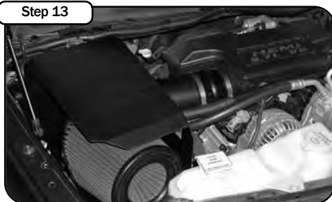
Place enclosed CARB EO sticker on a clean/smooth surface on or near the intake system. EO identification label is required in passing the Smog Check inspection. Your installation is now complete. Tighten all connections and clamps. Re-check after a few hours.
