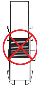
Not OK, threads are showing.
