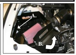
7. A.) There are two tabs on the Quick Fit Panel, insert the one closest to the headlight first into the slot on the factory airbox. B.) Next, carefully rotate the Quick Fit Panel counterclockwise until the factory clips line up with the tabs on the Quick Fit Panel. Make sure filter tab retains the Airaid Premium Filter. Now lock down the panel with the factory clips.
