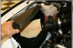
**2.** Remove the lid by lifting, and sliding it out of the tabs on the side of the airbox.
