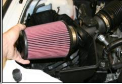
**5.** Install the Airaid Premium Filter on the factory intake tube.
