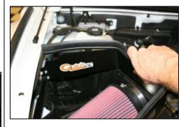
8. Starting at one end of the Quick Fit Panel, install the weather strip as shown.
