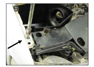
**6.** Using a 13mm socket, remove the factory
