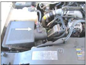
**2.** Disconnect the Mass Air Flow (M.A.F.) sensor and remove the factory airbox.Rock the factory air box back and forth and remove it from it's mounting. It is held in place with grommets. in,
