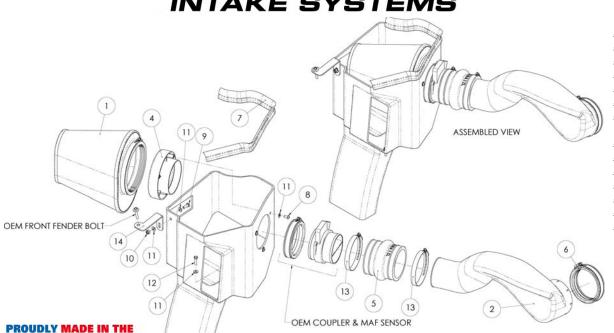
**Installation Instructions Part Number 200-247** 1999-06 GM Full Size SUVs and Trucks 2007 GMC Sierra "Classic" Truck 4.8L, 5.3L, 6.0L With Mechanical Cooling **Fan and Low Profile Hood**
