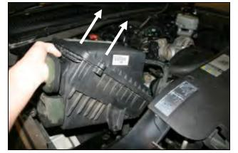
**4.** Rock the factory air box back and forth and then lift straight up remove it from the vehicle. There are only grommets holding it in, no bolts.
