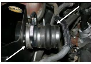
$\bf 9.$  Reinstall the  $\bf MAF$  sensor and coupler onto the filter adapter and tighten the clamp.
