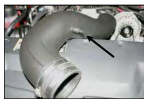
**14.** Install the 1/4" NPT x 3/8" Barb Fitting (#12) into the Airaid Intake Tube as shown. Next install the Urethane Coupler (#6) onto the throttle body end of the tube using two #64 hose clamps (#11). Only tighten the Tube side clamp at this time.
