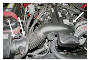
**4.** Loosen three hose clamps. One at each end of the factory intake tube, and one on the Mass Air Flow sensor (MAF) where it clamps to the factory airbox
