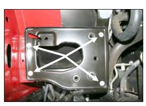
**8.**Using a 10mm socket, remove four bolts, and then remove the factory airbox mounting plate from the vehicle and set aside. Three of these bolts will be reused in step 11.
