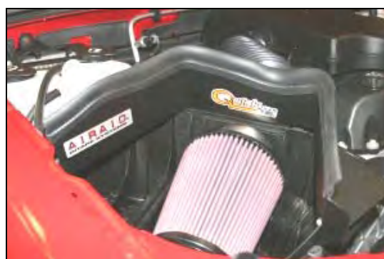
8. Install the provided weather strip (#4) on the top of the Quick Fit panels. For ease of installation, start next to the fender and work your way towards the front of the vehicle.
