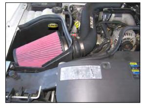
**15.** Install the Airaid Premium Filter (#1) onto the filter adapter, and tighten the hose clamp. Install the weather strip (#7) onto the Airaid Cold Air Box. Reconnect the **M.A.F.** sensor . (*Note: Start from one corner and work your way around to insure proper alignment of the weather strip.*)
