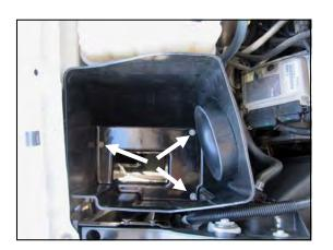
5. Install the Airaid Cold Air Box into the vehicle
