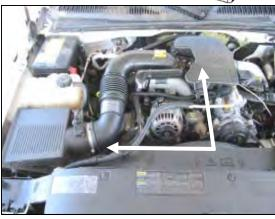
**1.** <u>Disconnect the negative battery cable.</u> Loosen the hose clamps on each end of the factory intake tube assembly and remove tube.
