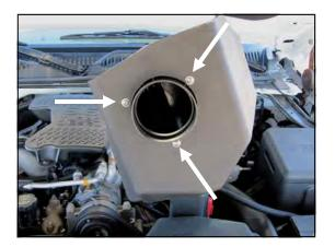
4. Install the Filter Adapter (#4) onto the Cold Air
