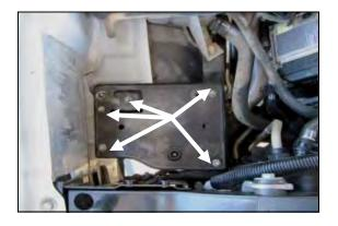
**3.** Using a 10mm socket, remove the five bolts and mounting plate from the engine compartment. Do not discard factory bolts. Three of them will be re used in step 5.
