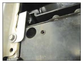
**7.** Install the Fender bracket (#13) as shown. **A**.) Secure the bracket to the fender using the factory bolt. **B**.) Use the 1/4-20 x 3/4" hex bolt (#14), one 1/4" flat washer (#9), and the 1/4-20 flange nut (#15) to secure the **CAB** to the Bracket. replacing the factory airbox. Secure the **CAB** using three of the bolts from step 3. Do not over tighten
