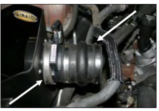
9. Reinstall the MAF sensor and coupler onto the filter adapter and tighten the clamp. Next install the hump hose (#5) onto the MAF using two #60 hose clamps (#13). Leave these two clamps
