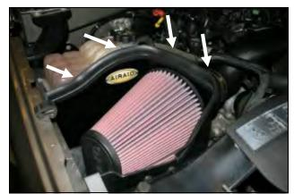
**12.** Install the provided weather strip (#7) along the top edge of the Airaid Cool Air Dam starting at the right fender working your way around towards the radiator. Install the Airaid Premium Filter (#1) onto the air filter adapter and tighten the hose clamp. Reinstall the factory beauty cover removed in step #1.
