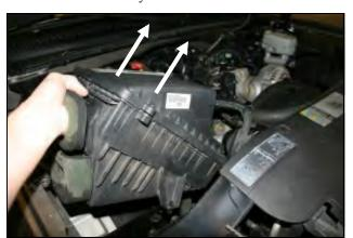
**4.** Rock the factory air box back and forth and then lift straight up remove it from the vehicle. There are only grommets holding it in place, no bolts.
