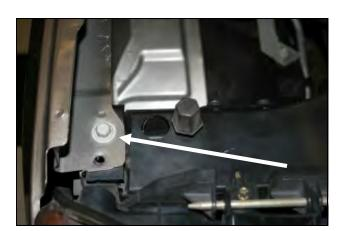
7. Remove the factory bolt that secures the right front fender to the radiator support. It will be reused in step #8.
