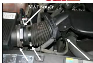
2. Loosen two hose clamps. One on each side of the Mass Air Flow (MAF) sensor.
