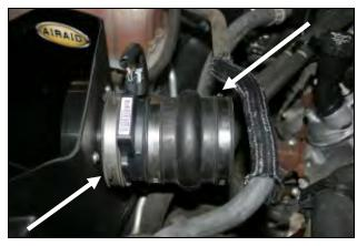
**9.** Reinstall the **MAF** sensor and coupler onto the filter adapter and tighten the clamp. Next install the hump hose (#5) onto the **MAF** using two #60 hose clamps (#13). Leave these two clamps loose for now.
