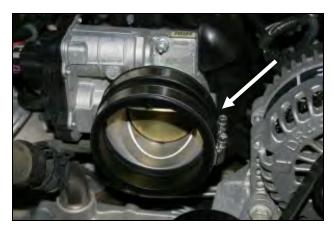
**10.** Install the provided coupler (#6) with two #64 hose clamps (#14) onto the throttle body. Do not tighten the clamps at this time.
