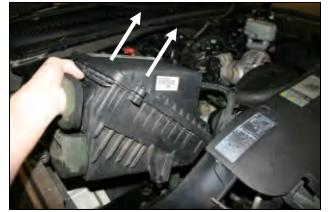
**4.** Rock the factory air box back and forth and then lift straight up remove it from the vehicle. There are only grommets holding it in place, no bolts.
