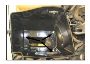
**6.** Install the Airaid **CAB** into the vehicle replacing the factory airbox. Secure the **CAB** using Three of the factory bolts from step 4. Do not over tighten
