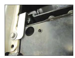
**8.** Install the Fender bracket (#13) as shown. **A.**) Secure the bracket to the fender using the factory bolt. **B.**) Use the 1/4-20 x 3/4" hex bolt (#14), one 1/4" flat washer (#9), and the 1/4-20 flange nut (#15) to secure the **CAB** to the Bracket.
