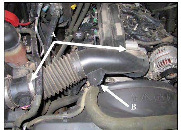
3.A.) Loosen the clamps securing the factory intake tube to the throttlebody and the Mass Air Flow Meter , or MAF. B.) Separate the hose anchor from the factory intake and remove the factory tube.
