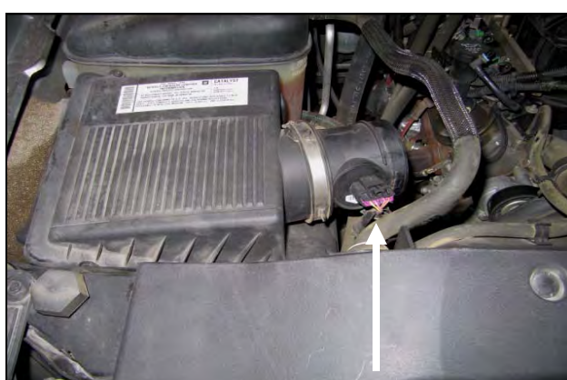
5. Disconnect the MAF sensor and remove the factory airbox and sensor from the vehicle. The airbox is secured to the vehicle with grommets and simply lifts out.
