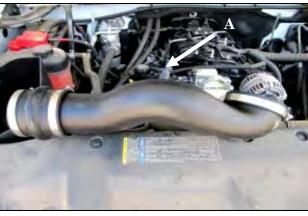
**11. A.**) Install the 3/8 NPT Fitting (#13) into the Airaid Intake Tube.
