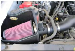
**14.** Install the Airaid Premium filter (#1) onto the Filter Adapter, and tighten the hose clamp. Install the Weather Strip (#8) onto the Airaid Cold Air Box. Reconnect the **M.A.F.** sensor. (<u>Hint</u>: Start from one corner and work your way around for ease of install.)
