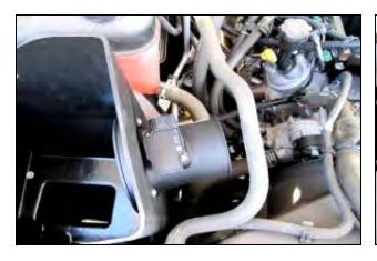
**10.** Transfer the Mass Air Flow sensor from the factory airbox into the Filter Adapter. Secure the sensor using the 8-32 Button Head Screws (#9).
