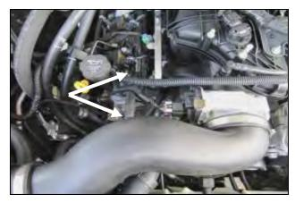
**12.** ) Install the 3/8" Breather Hose (#7) onto the Barbed Fitting and factory hard line.
