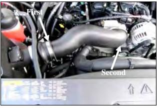
**11.** Install the Airaid Intake Tube assembly onto the Filter Adapter first, and then onto the throttlebody. Adjust for fit, and tighten all hose clamps. Reinstall the hose anchor into the Airaid Intake Tube.
