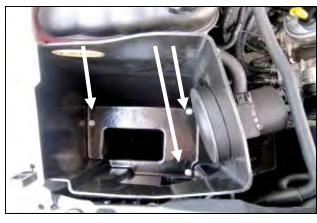
**9.** Install the **CAB** (#3) into the engine compartment and secure using three of the tray bolts from step **6.**
