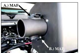
8. Install the Filter Adapter (#4) onto the Cold Air Box or CAB (#3) as shown using the three 1/4-20 Button Head Screws (#10) and 1/4" Flat Washers (#12).
