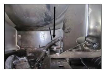
**7.** Secure the wiring harness to the inner fender as shown using the Edge Clip Cable Tie (#15).
