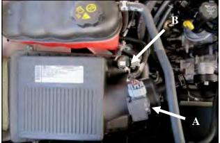
Disconnect the Mass Air Flow or MAF sensor (A) and the Manifold Absolute Pressure or MAP sensor (B) Remove the factory airbox from the vehicle.
