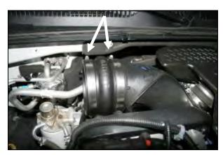
**5.** Install two #72 hose clamps (#10) onto the urethane hump hose (#4), and then slip the hump hose onto the end of the factory turbo intake tube as shown. Leave the clamps loose for now.
