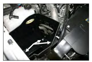
**4.** Install the Airaid Cool Air Box (CAB) (#3) into the vehicle as shown, replacing the factory air filter. Install three M6-1 x 25mm bolts (#9), and three flat washers (#7) thru the bottom of the CAB and into the factory captured nuts. Leave the bolts loose for now.
