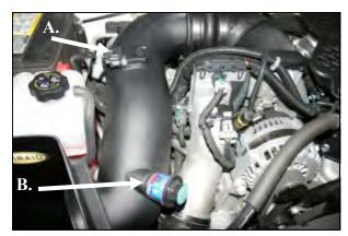
7. A.) Reinstall the Mass Air Flow sensor into the Airaid Intake Tube using two 8-32x 3/8" button head screws (#8). **Do Not Use The Factory Screws!**B.) Next, reinstall the factory filter minder and grommet into the Airaid Intake Tube.
