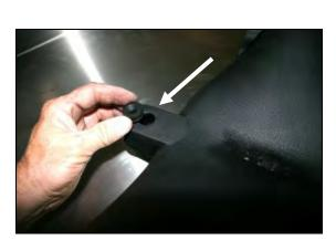
**8.** Install the two factory grommets that were removed in step #4, into the Airaid Intake Tube as shown
