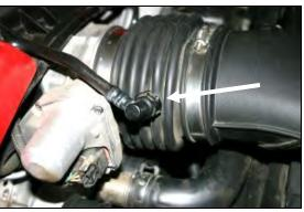
**2.** Push the tab on the top of the crankcase breather connector, and disconnect the breather hose from the factory intake tube breather fitting.
