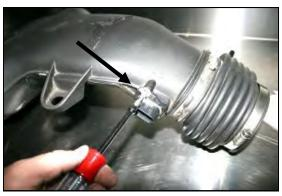
**5.** Using an IPR20 Torx Plus Security Bit (Or Equivalent) remove the two factory screws that hold the **MAF** sensor into the factory intake tube. Remove the **MAF** sensor for reinstallation in step #0
