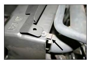
13. Slide one clip nut (#10) over the outside end of the plastic radiator cover and align it with the hole in the air dam. Install one rubber washer (#11) over the threads of the clip nut, and then align the air dam hole over the washer. Add one more rubber washer, one #8 flat washer (#9), and one 8-32x1/4" button head bolt (#8) to secure the air dam. Repeat this step on the passenger side. Refer to the line drawing on page one.
