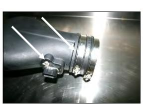
7. Reinstall the Mass Air Flow sensor removed in step #4, into the Airaid Intake Tube using two 8-32x3/8" button head bolts (#7).
