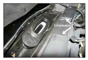
10. Set the Airaid Premium Filter into the area in front of the radiator. It will be mounted in step #
