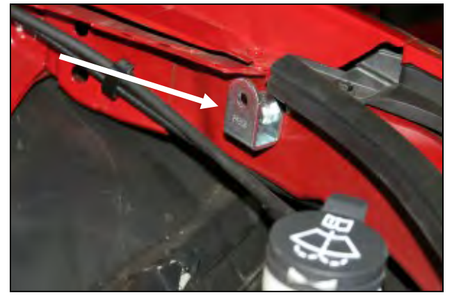
12. Replace the ground lug from step #11 with the side bracket (#23) as shown using one 6mmx12mm hex bolt (#14), and lock washer (#12).
