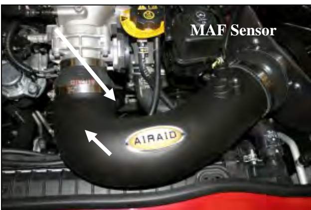
16. Install the Airaid Intake Tube (#2) into the hump hose first, and then into the reducing coupler. Adjust for fit, and tighten all four hose clamps.
