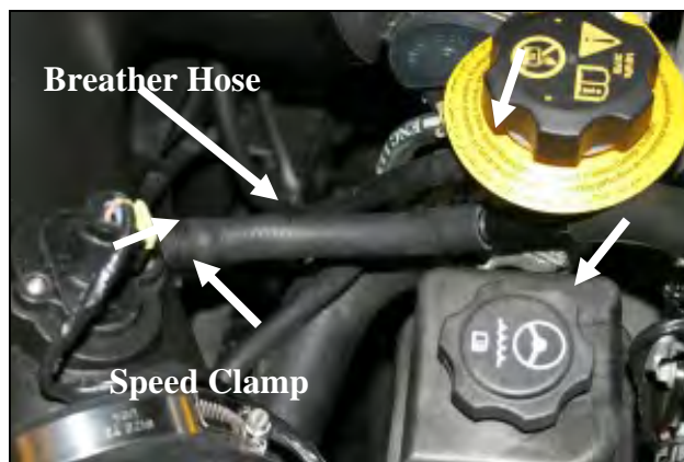
17. Install the 1/2"x 6" breather hose between the nipple on the air intake tube and the hard plastic crankcase breather tube. Refer to step #2. Install one #16 speed clamp (#20) over the breather hose at the nipple as shown.
