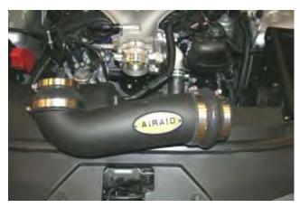
11. Install the Reducer Coupler (#8) onto the 90 deg. Bend of the Airaid Intake Tube (#2) and place and the Hump Hose on the opposite end as shown. Secure the couplers to the Intake Tube using the two #64 clamps (#22). Place the #48 clamp(#24) on the reducing coupler and the remaining #52 clamp(#23) on the Hump Hose.
