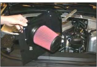
**12. A)** Install the Bracket (#25) on to the Rear Panel (#4) as shown using one 1/4-20 Button Head Screw (#15), 1/4" Flat Washer (#16), and 1/4" Serrated Nut (#17).**B)** Complete the assembly by attaching the Airaid Premium Filter (#1) Mass Air Flow Sensor.
