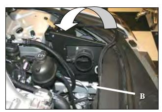
**13. A)** Lower the Airaid Performance Air box assembly into the engine cavity. Insert the Well Nut into the Factory core support grommet and rotate the assembly rearward until the bracket rests on the shock tower and the MAF panel's lower tab hole is lined up with the Tapped Chassis bolt hole. **B)** Secure the assembly by using the 1/4-20x 1/2 Bolt(#15).
