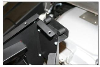
**6.** Attach the OEM Cover Bracket (#7) to the Rear Panel a shown using the remaining two sets of 6-32 hardware.
