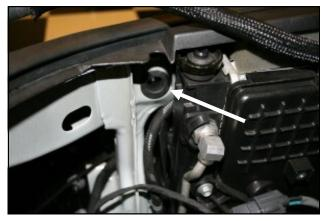
**4.** Use caution not to loose the factory core support grommet while removing the airbox assembly. It will be
