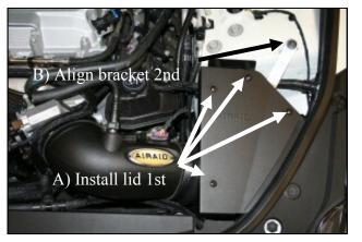
**13. A)** Attach the Edge Trim (#27) on the Cover (#6) as shown and install the cover using the four Black 1/4-20 Phillips Head Screws. **B)** Line up the Bracket with the fender bolt hole and secure using the factory hardware. **Note: Steps must be performed in order to avoid difficulty with aligning bolt holes.**
