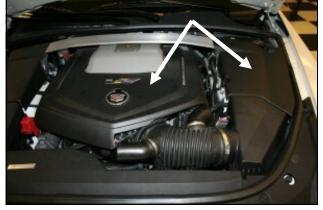
1. **Disconnect the negative battery cable.** Remove the engine and shock tower covers by simply pulling up on them and sliding out from the vehicle. These will be reused later in step 14.
