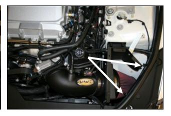
**12.** Install the Airaid Intake Tube (#2) assembly onto the filter Adapter first, and then onto the throttlebody. Adjust for fit, and tighten all 3 hose clamps. Next reconnect the **MAF** sensor and Breather line. Slide the Edge Clip Cable Ties (#30) about 6" apart along the fender pinch weld and return the coolant line to it's original location. Secure the coolant line using the cable ties and trim off excess.
