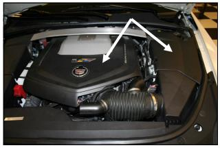
1. <u>Disconnect the negative battery cable.</u> Remove the engine and shock tower covers by simply pulling up on them and sliding out from the vehicle. These will be reused later in step 14.
