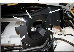
**5.** Install the Adapter Panel (#5) to the MAF Panel (#3) as shown using four 6-32 screws (#12), 6-32 Kep nuts, and #6 flat washers (#14). Attach the Rear panel (#4) to the MAF panel using two 6-32 screws.
