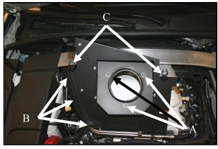
8. A) Install the Filter Adapter onto the MAF panel using three 1/4-20 Button Head screws (#17) and 1/4" Flat washers (#18). **B)** Attach the Weather Strip (#11) to the curved edge of the MAF Panel. C) Insert the 5/8" hose anchors (#29) into the two horizontal tab holes on the MAF panel
