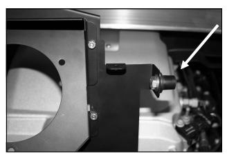
7. Attach the 5/8" Well Nut (#23) to the vertical MAF Panel tab as shown using the 5/16 Hex Bolt (#21) and the 5/16" flat washer (#22).
