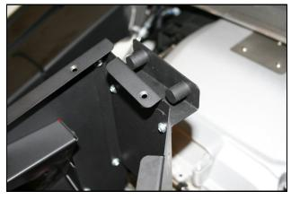
6. Attach the OEM Cover Bracket (#7) to the Rear Panel a shown using the remaining two sets of 6-32 hardware.
