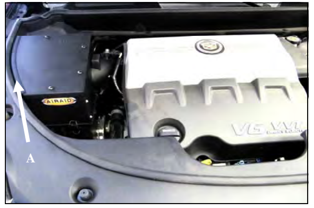
13. A) Attach the Weather Strip (#7) to the curved edge of the Top Panel (#5). B) Attach the Top Panel to the Airaid Performance Airbox using the four 1/4-20 Phillips Head Screws. Reinstall the engine cover and the oil fill cap.
