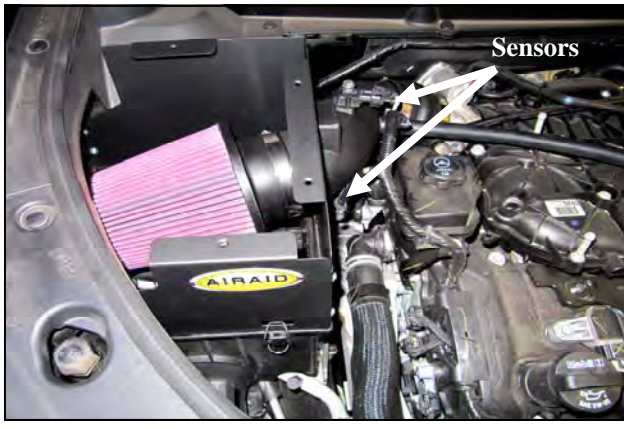
12. Install the Airaid Premium Filter (#1) to the Intake Tube. Reconnect the Mass Air Flow and MAP sensors.
