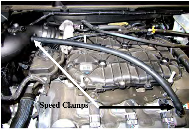
11. Attach the 1/2" Breather Hose to the Intake Tube nipple and the factory valve cover fitting. Secure using the Speed Clamps (#17).
