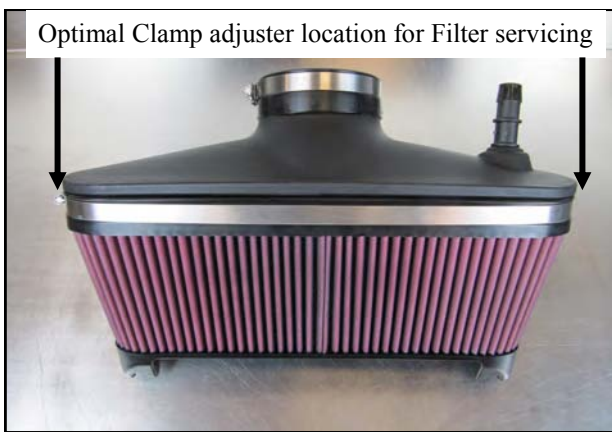
5. Create the Filter Assembly as shown by mounting the Filter onto the filter Base and securing it with the Large Clamp. Slide the small clamp on to the air outlet and insert the Grommet and Barbed Fitting into the breather port.
