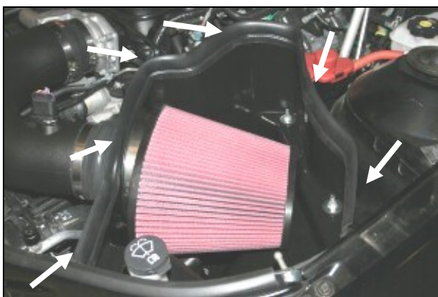
17. Install the Airaid Premium Filter onto the filter adapter and tighten the clamp. Next install the weather strip onto the top of the CAB. For ease of installation, start the front of the CAB near the radiator and work your way around towards the fender. Reinstall the engine cover and oil fill cap.
