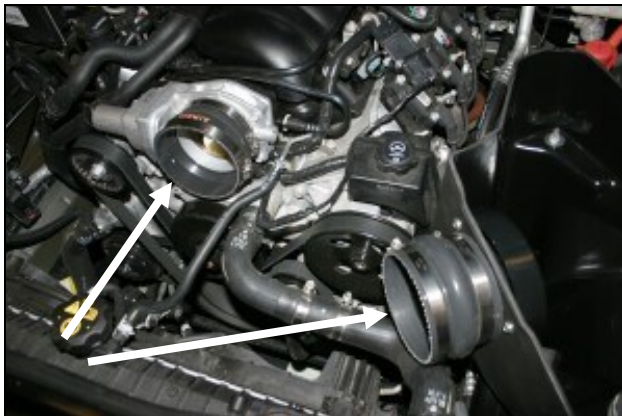
14. Install the hump hose (#5) onto the filter adapter using two #64 hose clamps (#9). Next install the reducing coupler (#6) with one #60 hose clamp (#11) on the throttlebody and one #68 hose clamp (#10) on the large end.
