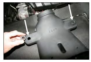
**6.** Install the factory grommets removed in step #5 into the Airaid intake tube (#2).
