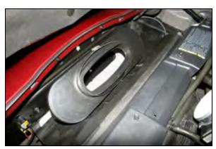
**8.** Install the Airaid Premium Filter into the area in front of the radiator. It will be attached to the Airaid intake tube in step #11.
