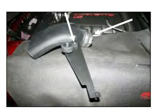
**4.** Reinstall the barbed fitting removed in step #3 into
