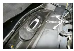
**10.** Set the Airaid Premium Filter into the area in front of the radiator. It will be mounted in step # 15.
