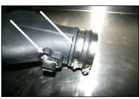
7. Reinstall the Mass Air Flow sensor removed in step #4, into the Airaid Intake Tube using two 8-32x3/8" button head bolts (#7).
