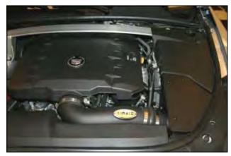
ble check your work! Make sure there is no foreign material in the intake path. Make sure all clamps, hoses, bolts, and screws are tight. Double check the hood clearance.
