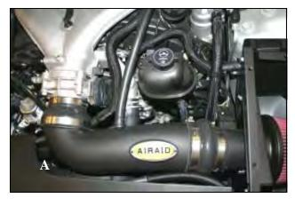
14.A) Install the Airaid Intake Tube assembly onto the Mass Air Flow Sensor first, and then onto the throttle body. Adjust for fit, and tighten the hose clamps. **B**) Replace the factory breather line on the valve cover with the 26" Airaid Breather Hose(#11). Secure the breather hose to the intake tube nipple using the black Speed Clamp (#29)
