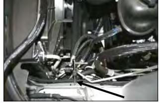
**5.** Locate the pre existing hole in the chassis and tap it for a 1/4-20 bolt. Use a 1/4-20 NC tap with anti-seize lube or equivalent, and follow the 1/4 turn forward, 1/2 turn back rule. This will ensure that clean threads will be cut into the hardened steel.
