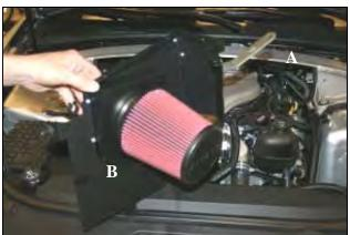
**12. A)** Install the Bracket (#25) on to the Rear Panel (#4) as shown using one 1/4-20 Button Head Screw (#15), 1/4" Flat Washer (#16), and 1/4" Serrated Nut (#17).**B**) Complete the assembly by attaching the Airaid Premium Filter (#1) Mass Air Flow Sensor.
