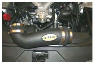
11. Install the Reducer Coupler (#8)onto the 90 deg. Bend of the Airaid Intake Tube (#2) and place and the Hump Hose on the opposite end as shown. Secure the couplers to the Intake Tube using the two #64 clamps (#22). Place the #48 clamp(#24) on the reducing coupler and the remaining #52 clamp(#23) on the Hump Hose.
