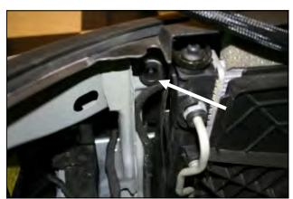
**4.** Use caution not to loose the factory core support grommet while removing the air box assembly. It will be needed in step **13**.
